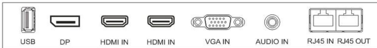
VGA INPUT: D-SUB 15 pins Connector
