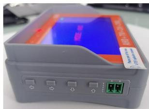
The tester incorporates the Pelco-D, / P etc. PTZ control protocol through its own RS485 interface.
