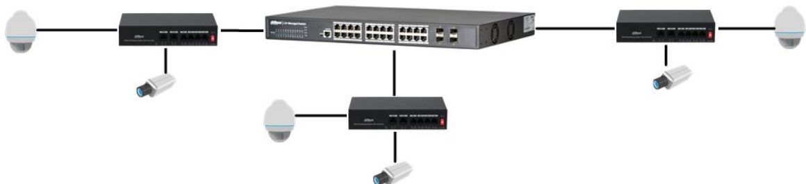
Figure 1-1 Typical networking scene Layer-2 Managed Switch
