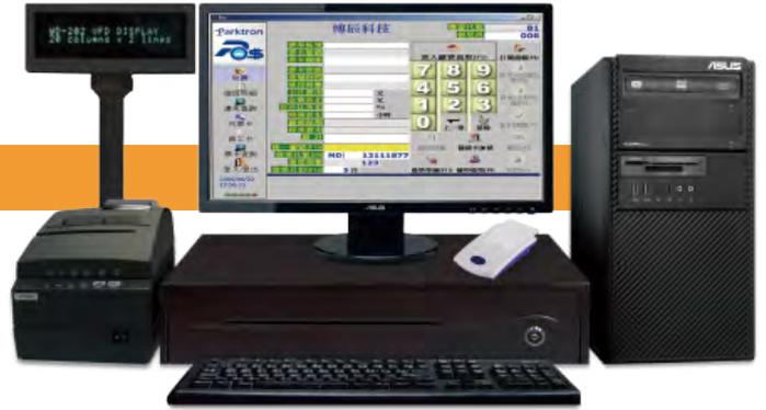
CCST209 Cashier Station is a PC based POS computer in CPS2000 parking system. It supports Chipcoins (Mifare® IC inside) as parking tickets and provides a manned payment service for a parking facility. In case of network disconnection, CCST209 can still be operated under stand-alone mode; off-line data will be saved and then sent back to Central Management Server after network reconnected.
