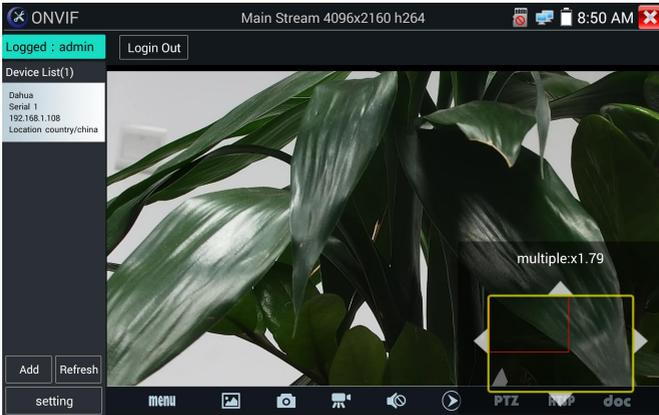
When the image is enlarged, if not operate on touch screen, it can operate by the keyboard ,press the key **TELE+** to zoom in , press the key **WIDE-** to zoom out ,press upward and downward key to move image.
