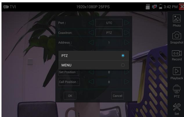
Input calling dome camera menu address code, after finishing the parameter settings, you can press the key **ENTER** or click the icon
