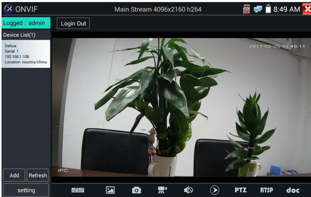
segments. It lists cameras name and IP address on the Left of screen. Tester can auto login camera and display camera image. Factory default use admin password to auto login, if you modified the password, then default use the modified password to log in.
