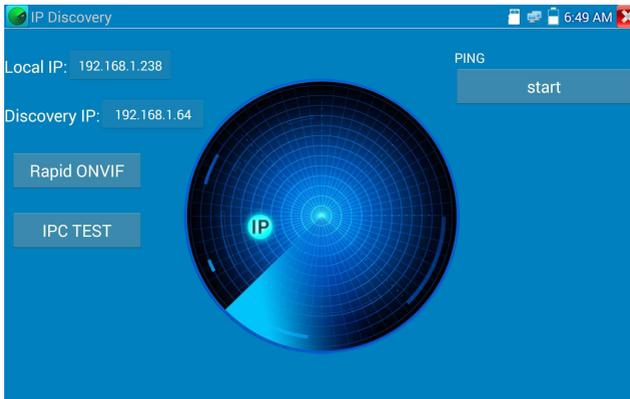
**Local IP:** Tester's IP address, Tester can auto-modify the tester's IP to the same network segment with the scanned camera's IP.
