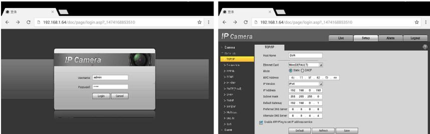
The IP camera and the tester be on the same network segment for the browser to interface with the camera. If they are not in the same segment, click the button
