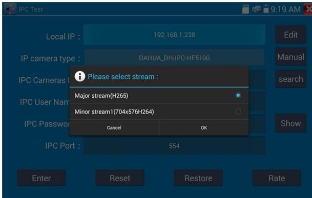
**IP Camera's IP:** Enter the IP camera's IP address manually or click "Search" to auto-scan for the IP camera's IP address. It is better to directly connect the IP camera to the tester so the search results will only display the camera's IP address. If the tester is connected to a PoE switch, it will find and display several IP address.
