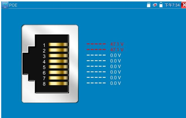
Connect a network cable from a PoE switch to the tester's PSE IN port. Connect an IP camera or other PoE using node to the tester's LAN port, the PoE voltage and the cable's pin connection status show on the screen.
