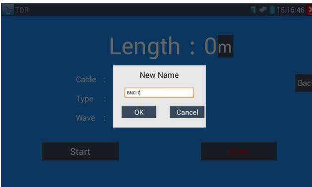
**Application:** TDR test is used for pulse reflection method, to transmit pulse signal for tested cable, when cable is open circuit or short-circuit, reflected pulse is generated, the tester receives and deals with the reflected wave, measurement results displayed on the screen. TDR can test cable open circuit and
